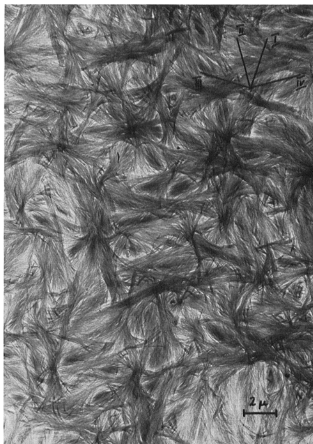
Fig. 7. Electron micrograph of an oriented Nylon 6 layer overgrown onto (001)-KCl with 4 favoured orientations 17 .
